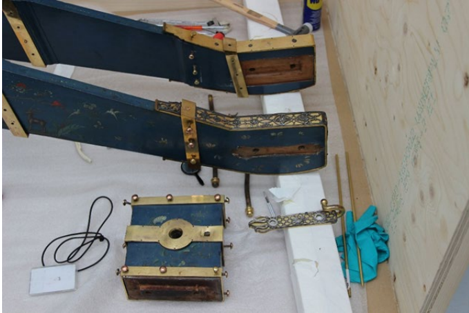
The wooden tailstock with the drawbar eye is very shallowly recessed between the two sides and the copper bolts are very thin. (Rijksmuseum, Amsterdam, Behandelingsrapport NG-NM-1015, 2012)
